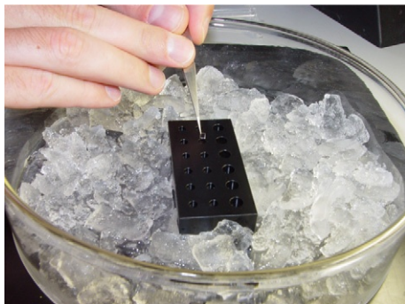
Figure 5.4 Placement of carbon film over a sample. A homemade plastic block with holes drilled into it, each with a holding capacity of about 25 \mu\text{l} , is precooled on ice, and 30 \mu\text{l} of a sample is loaded into one hole. A thin carbon film is floated off a mica support by holding the mica with forceps and placing it into the sample at a slight angle. Once the carbon film is released, the mica is removed, and macromolecular complexes are allowed to adsorb for the appropriate time.
